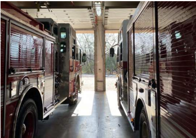
FIGURE 9: The apparatus bay doors are undersized for modern equipment, making for difficult entry and exit while responding to a call.
