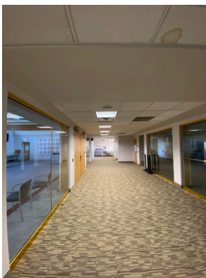
City Hall Figures 3 and 4 Council Chamber Hallway/Waiting and Physical Development Waiting Area While the corridor immediately adjacent to the City Council Chambers is wider than average, there is no seating, and gatherings in the hallway are both visually and acoustically distracting through the full-height non-acoustic glass partitions into the chambers. A 2019 renovation reconfigured the service counters at Physical Development, providing a modest waiting area where there was previously none. Photo taken October 2020 when City Hall was largely closed to the public.
